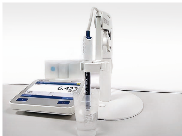
Figure 2. Measurement of conductivity sample using InLab 710.
