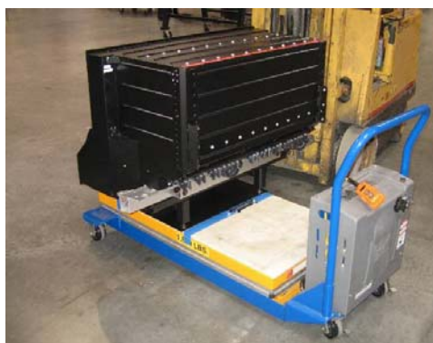
Figure 1 – Tesla Roadster battery pack
