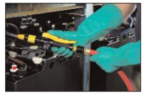
To fill the batteries, a hose is attached to the input fitting and a valve is opened. The water flows through the plastic tubing and, simultaneously, into each of the cells. Within 15 to 20 seconds, the battery is filled with each cell receiving the precise amount of water needed.
