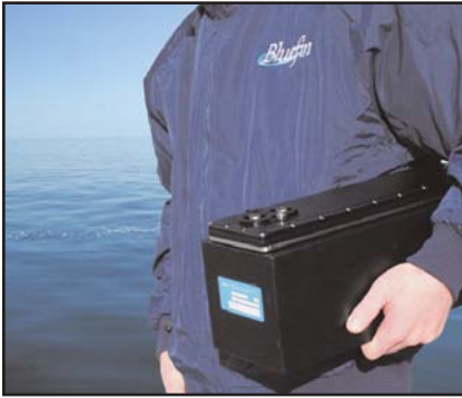
Figure 2 Free from cumbersome pressure chambers, the Bluefin 1.5kW-hr battery pack is easily swapped out of vehicles.
