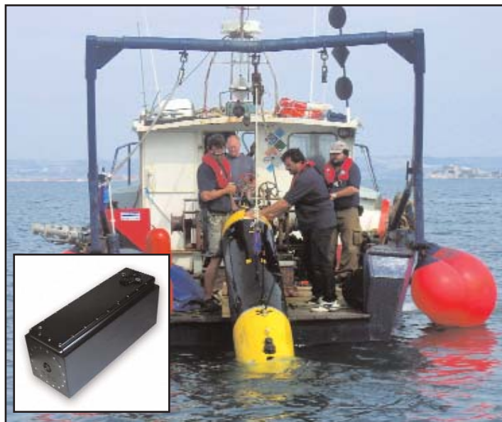
Figure 1. Operators bring on deck the Bluefin-21 AUV at the end of its mission. The vehicle carries out missions to ocean depths of 4,500 meters, and uses li-poly pressure-tolerant battery technology. (Bottom left) the 1.5 kW-hr battery pack which powers many AUV systems.
