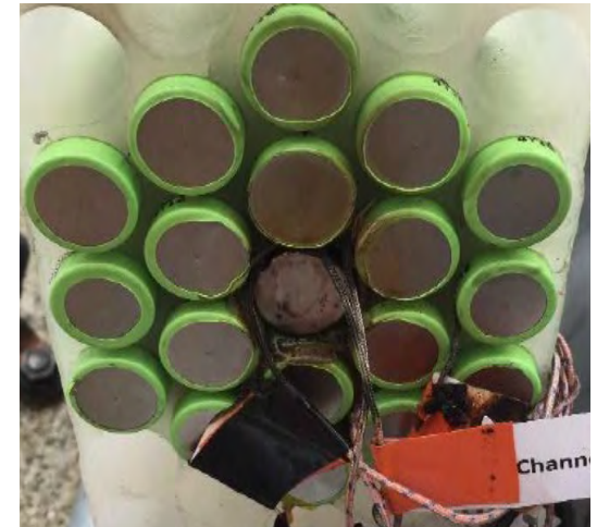
Negative side after thermal runaway event
