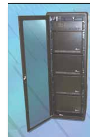
Figure 2. International Battery's lithium ion battery modules with battery management system (BMS) that is integrated into a standard 19-inch portable rack mount chassis and enclosure (see Figure 2). As with the CES project, large-format Li-Ion batteries were chosen because of their proven high-energy density, robust thermal and cycling performance as well as easy system expandability.
