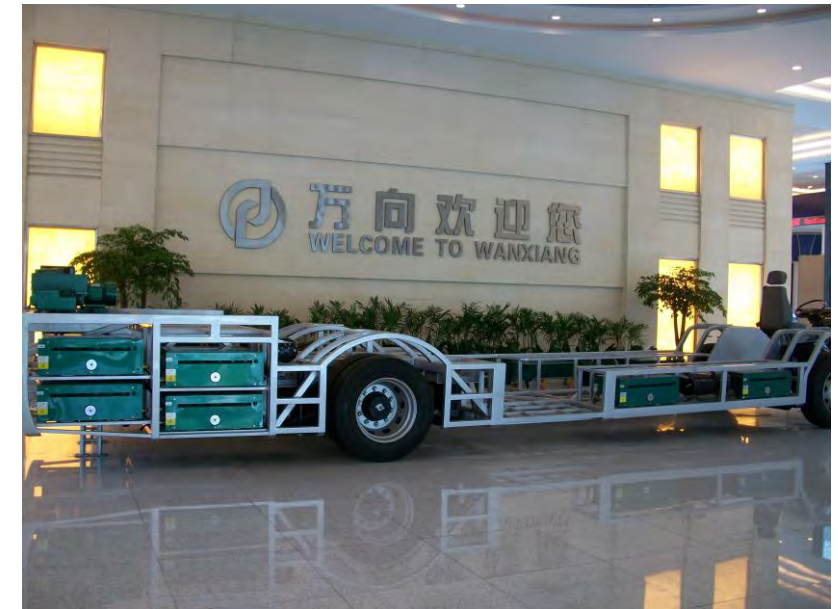
Wanxiang E-Bus drivetrain and chassis with LFP batteries. Source: China-EV.org
