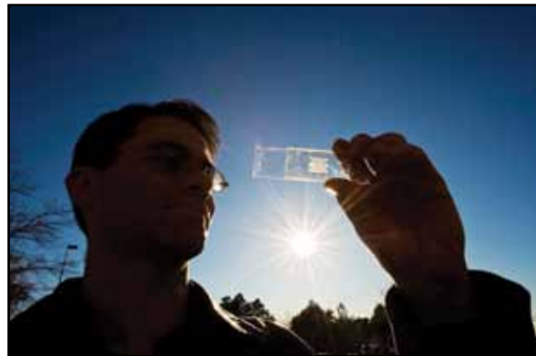
Sandia project lead Greg Nielson holds a solar cell test prototype with a microscale lens array fastened above it. Together, the cell and lens help create a concentrated photovoltaic unit. (Photo by Randy Montoya)
