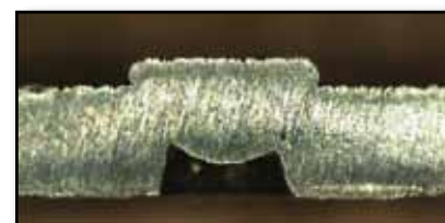
Figure 3. Projection Weld Cross-section (35X magnification)
