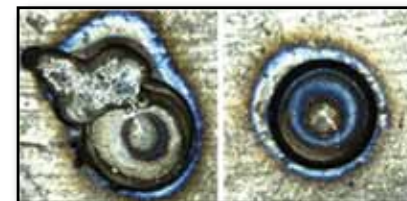
Figure 2. Projection Weld Top Views, Expulsion (left) No Expulsion (right)
