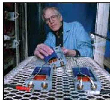
Argonne researcher Ira Bloom prepares GS-Yuasa high-power, lithium-ion batteries for testing. Photo courtesy of Argonne National Laboratory.
