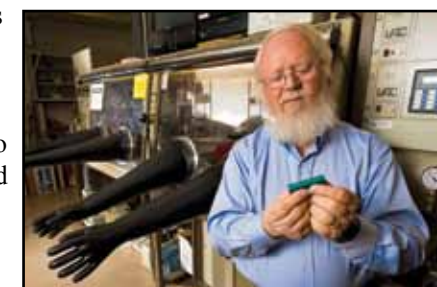
Sandia researcher Pete Roth examines a lithium-ion battery before dismantling it for testing in the chamber behind him. Photo by Randy Montoya
