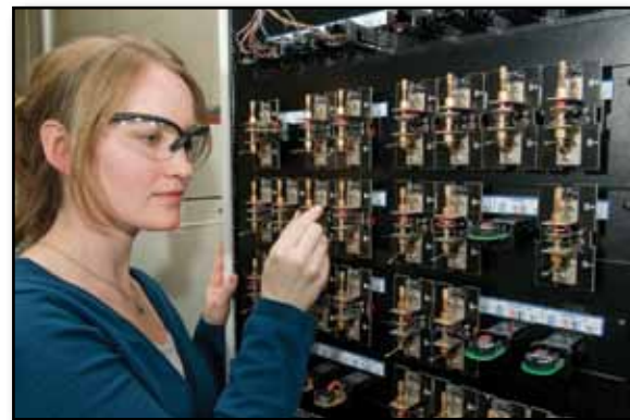
Argonne researcher Lynn Trahey loads a coin-sized cell on a testing unit used to evaluate electrochemical cycling performance in batteries. Photo by Wes Agresta / Courtesy Argonne National Laboratory.
