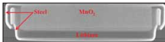
Figure 1. CR2050 lithium/manganese dioxide primary cell ~100 percent SOC.
