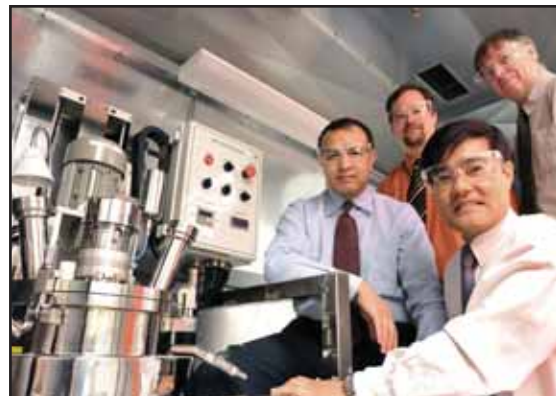
Argonne National Laboratory battery researchers (from left) Khalil Amine, Chris Johnson, Sun-Ho Kang and Mike Thackeray flank a continuously stirred tank reactor used to produce scaled-up quantities of cathode materials for lithium-ion batteries.
