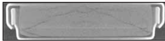
Figure 2. CR2050 discharged lithium/manganese dioxide primary cell ~0 percent SOC.
