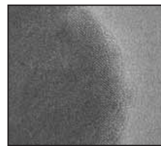
Scanning electron micrograph of a particle of the MIT battery material reported in Nature. Dark area indicates the inside of the particle surrounded by a lighter surface layer only five nanometers wide. Photo Courtesy of Ceder Lab/MIT.
