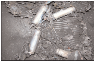
Figure 1. Remnants of an overcharged Li-Ion battery pack.
